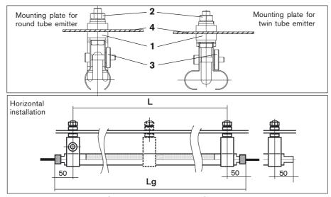
Mounting dimensions: L = Overall length of emitter LG - 2x50 mm
